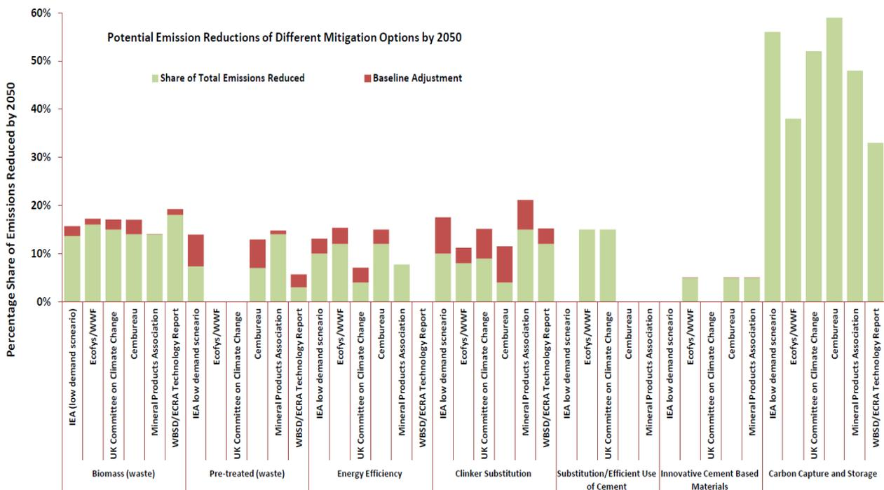
Figure 3: CO<sub>2</sub> mitigation potential estimated by different cement roadmaps (compiled by DIW, Berlin)
